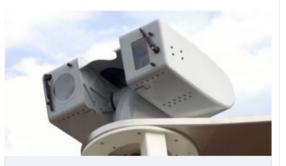
By integrating CCTV cameras and other electrooptical sensors such as thermal imagers into the Sea Cobra platform, the system can be tailored for a range of uses on fixed and floating platforms.
